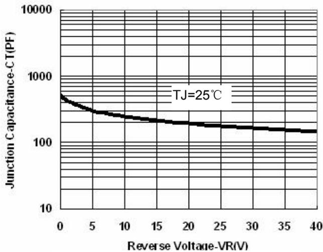
Fig.1-Typical Junction Capacitance
